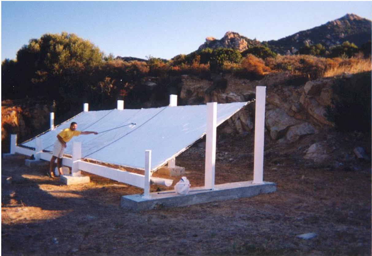
Figure 10 – Big OPUR Dew Condenser in Corsica
